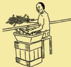
Bins are easier to reach if they are beside you at waist height or close to your elbow
